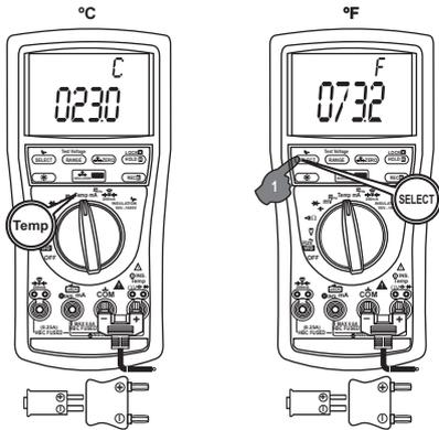
**Note :** Be sure to insert the banana plug type-K temperature bead probe Bkp60 with correct + – polarities. You can also use a plug adapter Bkb32 (Optional purchase) with banana pins to type-K socket to adapt other standard type-K mini plug temperature probes.
