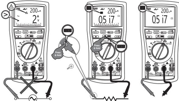
**Lock-Test mode** is recommended for continuous measurement. To apply, press the **LOCK** button momentarily to display the annunciator **LOCK** before pressing the **TEST** button momentarily. The LCD will show both **LOCK** & **TEST** to indicate continuous measurement is active. Press again either button momentarily to release the Lock-Test mode.
